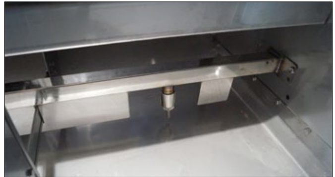
Water comes out of the press valves in the trough.
